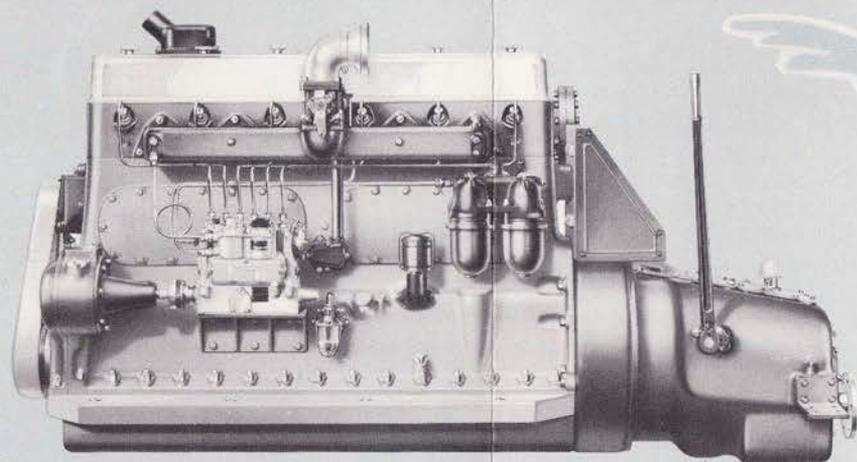
*LEFT—Fuel injection side of Defender and Rolute series marine engine with 2:1 reduction and reverse gear. Rated at 160 and 175 hp. respectively, these Waukesha-Hessselman Oil Engines have all the advantages of low pressure construction: integrally cast cylinder frame and crankcase, wet sleeve cylinders, overhead valves, full pressure oiling, and patented Waukesha non-stick piston rings. Like all Waukesha Marine Engines, they incorporate a special closed cooling system.*
